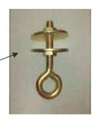
**Step 2:** Large fender washer should be installed against the hutch on the outside. Next, add a lock washer. A nut should be installed on top of the lock washer. This helps adjust the eyebolt out to the correct distance (approx. 1.5" to the center of the eye on the top and 1.75" to the center of the eye on the bottom).
