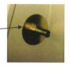
**Step 4:** Fence is locked into position when the upper eyebolt and the lower eyebolt are within one section on the fence. This keeps the fence from moving forward and backward.
